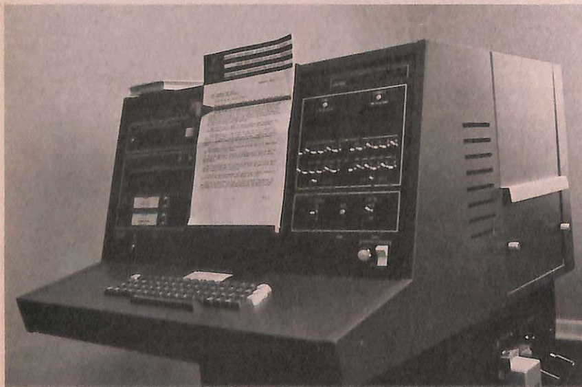
The Compugraphic Compuwriter II is the first piece of equipment purchased from the Capital Funds Campaign. It enables the Advocate to set its own type and furnish the printer with camera-ready copy.
